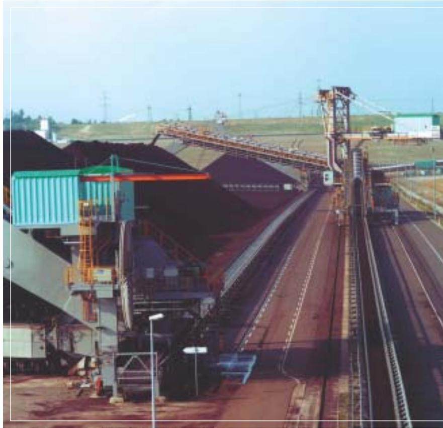
with this capacity have not been used in the German brown coal industry before. Each unit can handle 1,800 t of raw brown coal per hour. All plants meet special requirements of noise and dust protection, since villages are located in the close surroundings. Thus, the overland belts were covered over, the coal blending stockyard was equipped with sprinklers which spray water on the stockpile, if necessary. The plants and equipment are controlled and operated from a central conveyor control room.
